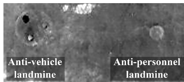
Figure 1- shows how a FLIR sUAS thermal camera can see AV and AP mines in long grass.
