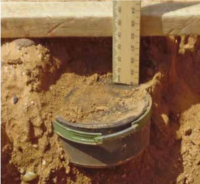
Photo 1. Above is a photo of one of the PMA-3 AP landmines that was identified in sUAS TIR imagery, with validation provided by deminers who excavated to show that it was buried at a depth of 4cm depth at a live, 30-year-old in situ minefield.
